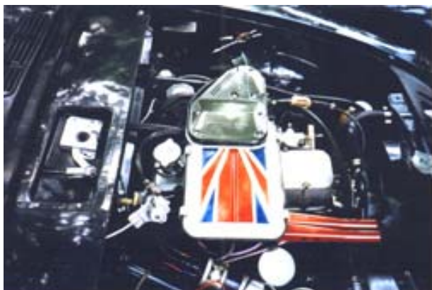
ABOVE: The Roots fiber pad type air cleaner assembly. Part No. 6601053 issued 1965.
